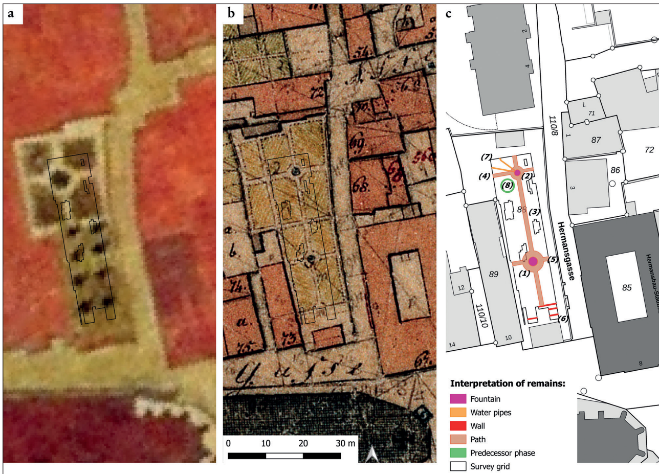
Fig. 5. Representation of the Baroque garden of the Hermansbau . – a. Map from 1737 displayed in the municipality of Memmingen; b. Map from 1819 (= Uraufnahme ). Black lines mark the outline of the GPR survey grid; c. GIS-based interpretation of the anomalies detected during the GPR survey.
