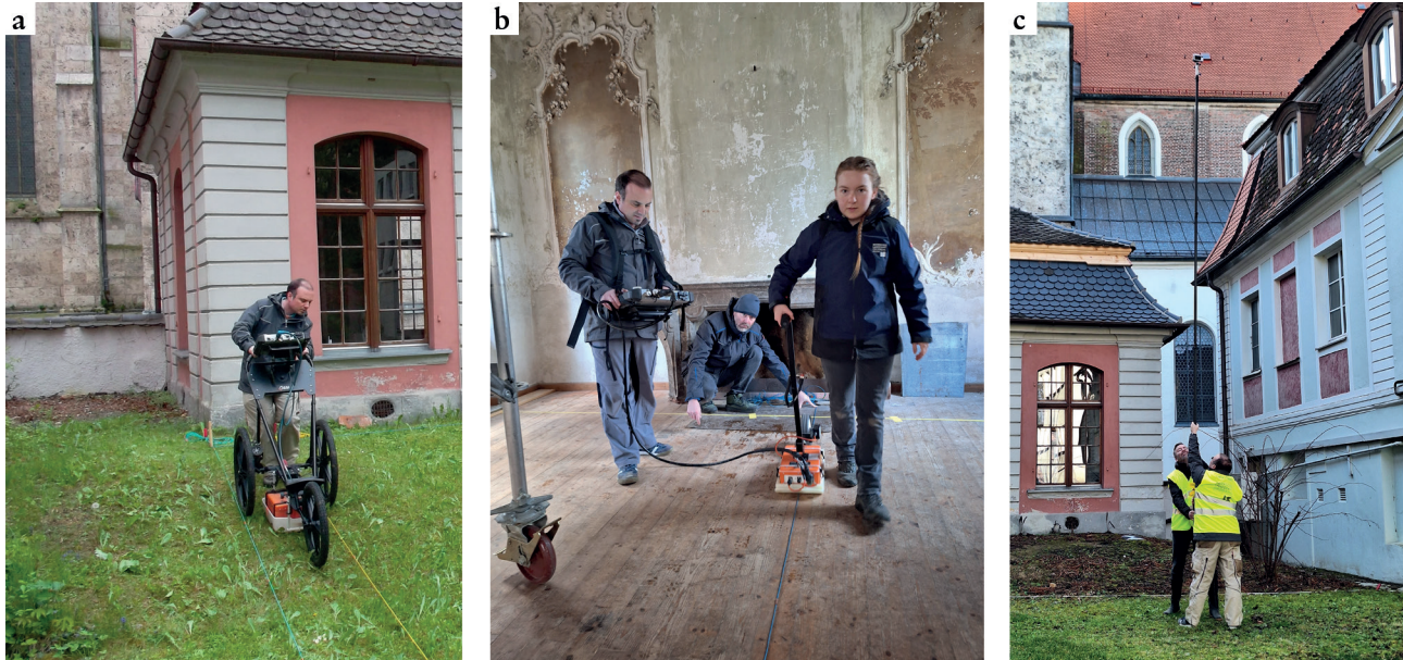
Fig. 2. Survey equipment utilised. – a. GSSI SIR-4000 with 400 MHz antenna for the survey of the Baroque garden; b. GSSI SIR-4000 with 900 MHz antenna for the survey of the cellar underneath the pavilion; c. SfM survey with Panasonic GX800 mounted on a high monopole (Photos: BLfD).
